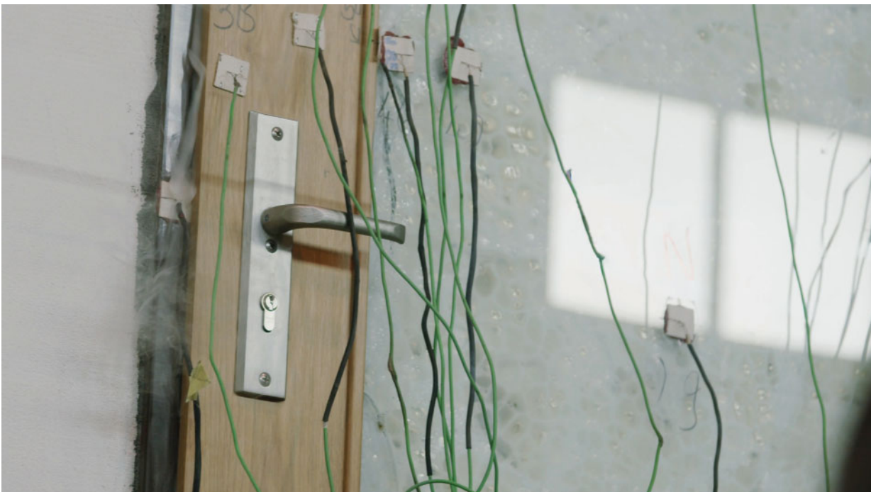
Doors during fire tests.
