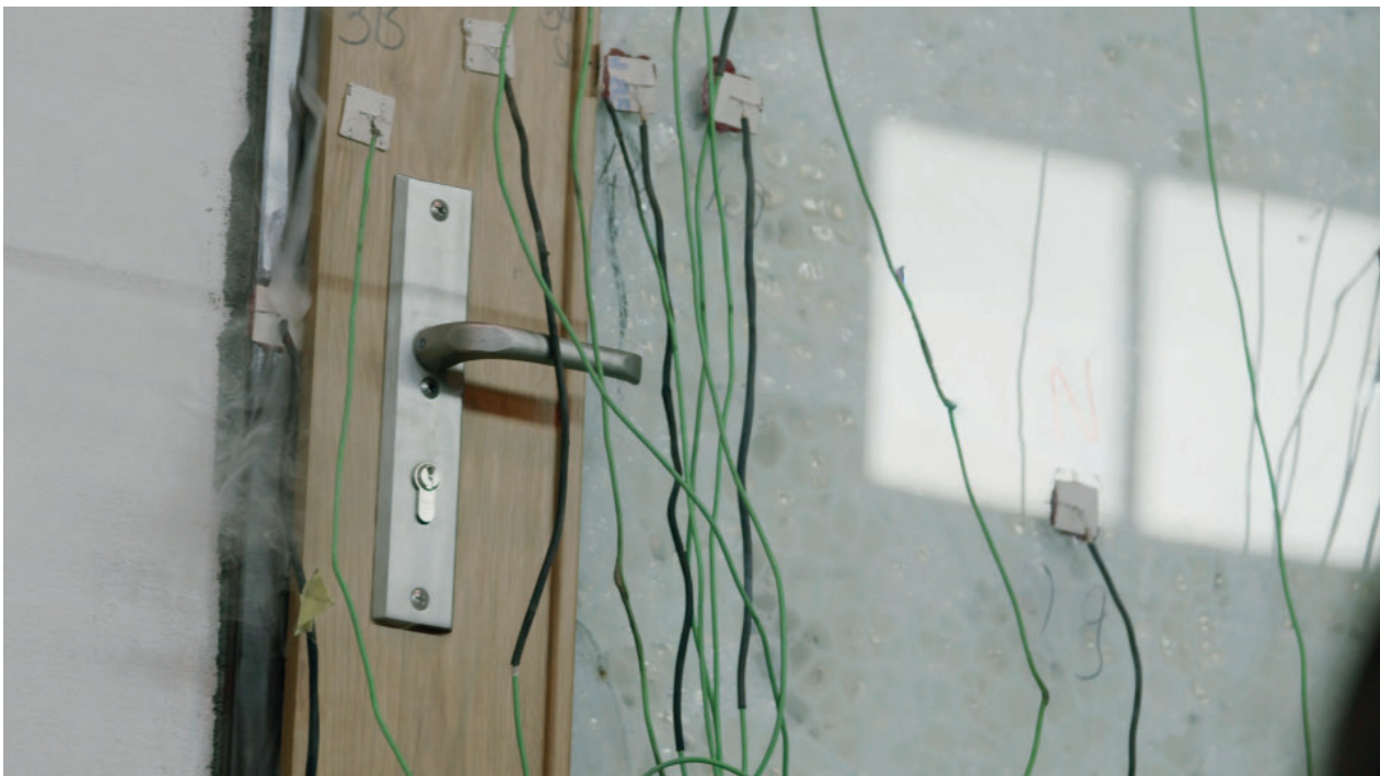
Doors during fire tests.
